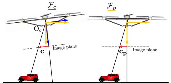
Fig. 8. Attitude compensation:  $\mathbf{c}$  is the position of the object that is estimated by the visual tracking algorithm, and  $\mathbf{c}_p$  is the corresponding position in the frame  $\mathcal{F}_p$  where the rotation has been compensated.
