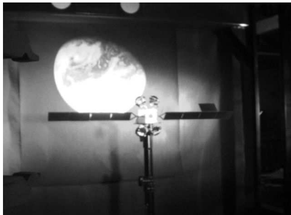
Fig. 11: Initial image for situation 1. The distance chaser/target is 1.55m (646m in the equivalent real space context).
