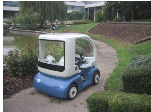
Fig. 12. CyCab autonomously drives on the narrow path in experiment 2.
