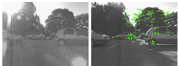
Fig. 15. Sun shines into the camera in the reference image (left) but not in the current image (right) during navigation in experiment 3.
