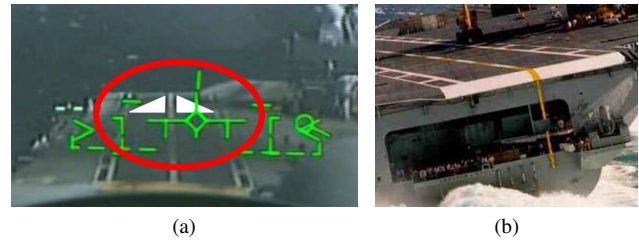
Fig. 1. (a) Pilots try to put the HUD velocity vector at the basis of the triangle mark in order to follow the glide slope; (b) The angle between the drop and the alignment lines (yellow and dash) provides lateral information
