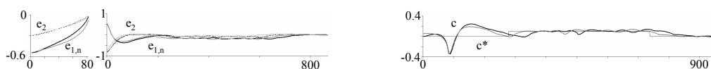
Figure 13: Variables for the second image-based experiment, with correct (black) and coarse (gray) calibration. Errors e_{1,n} (solid, dimensionless), and e_2 (dotted, in rad), with RCC (left) and BRC (center). Applied (thick) and desired (thin) curvatures (right, in \text{m}^{-1} .)
