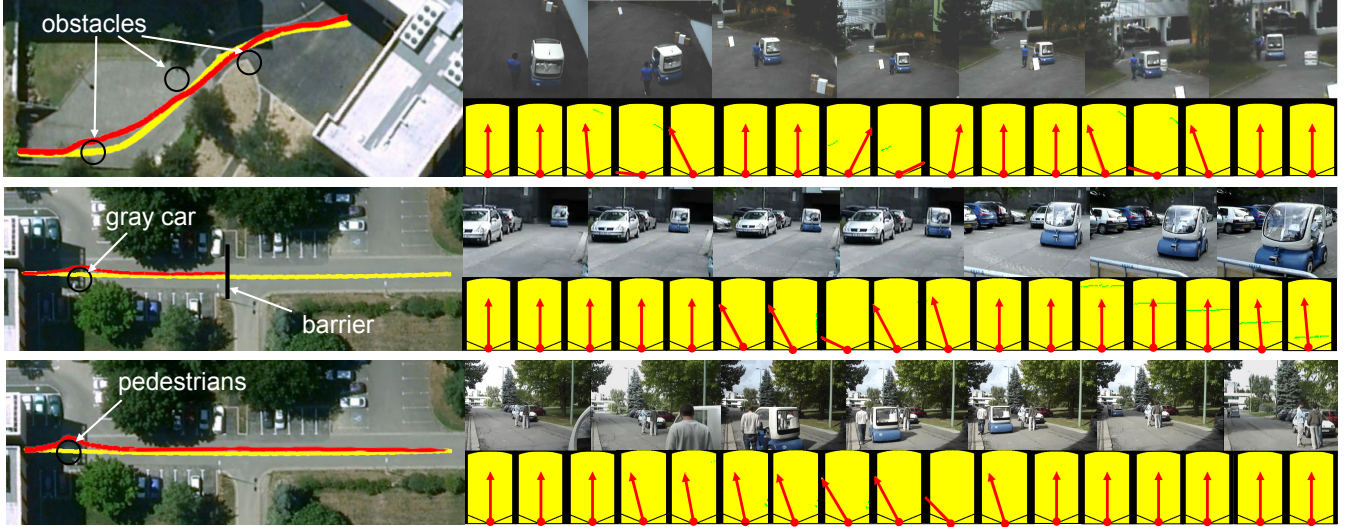
Fig. 3. Top to bottom: experiments 1 to 3. Left: reconstruction of the replayed path with (red) and without (yellow) obstacles. Right: snapshots (above) and grids (below) in the presence of obstacles. The red vectors show the orientation of f .
