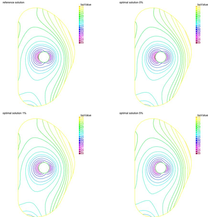
**Figure 4.** First test case (TC1),  $u_{ref}$  given by Eq. (38). Top left : reference solution  $\psi_{N,ref}(u_{ref}, g)$ . Top right : recovered solution with no noise on the data. Bottom left : recovered solution with a 1% noise on the data. Bottom right : recovered solution with a 5% noise.
