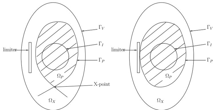
**Figure 2.** The plasma domain  $\Omega_P$  and the vacuum region  $\Omega_X$ . The plasma boundary is determined by an X-point configuration (left) or a limiter configuration (right). The fictitious contour  $\Gamma_I$  is represented inside the plasma.
