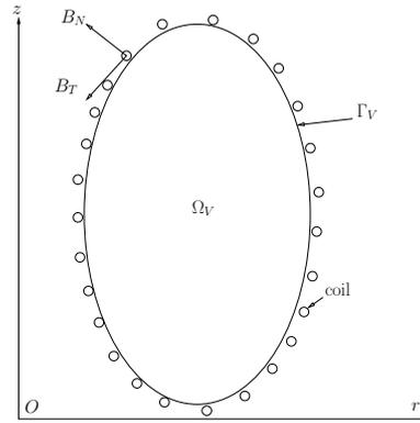
**Figure 1.** Cross section of the vacuum vessel : the domain  $\Omega_V$ , its boundary  $\Gamma_V$ . Coils providing measurements of the components of the magnetic field tangent and normal to  $\Gamma_V$  are represented surrounding the vacuum vessel.
