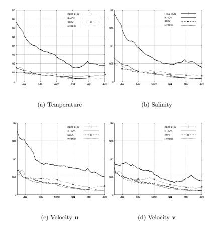
**Fig. 2** Absolute Rms error obtained by each method during the first 6 months of simulation, at 15m. depth. Solid line with +: free run, solid line: R-4D-Var, dashed line with o: SEEK filter and dashed-dotted line: hybrid method.
