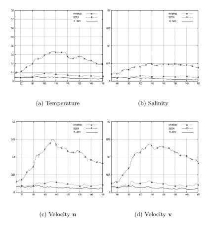
**Fig. 5** Rms error the last 6 months of simulation, at 15 m. depth, in the eastern part of the basin. Solid line: R-4D-Var, dashed line with o: hybrid method and dashed-dotted line with x: SEEK filter.
