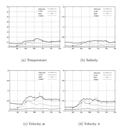
Fig. 6 Rms error the last 6 months of simulation, at 15 m. depth, in the western part of the basin. Solid line with +: free run, solid line: R-4D-Var, dashed line with o: SEEK filter and dashed-dotted line: hybrid method.
