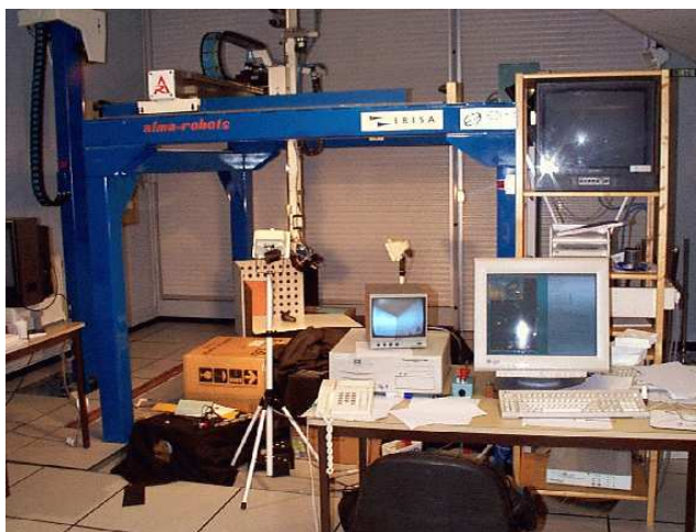
Figure 11: Experimental setup at IRISA-INRIA Rennes: six degrees of freedom cartesian robot with a camera mounted on the end-effector.
