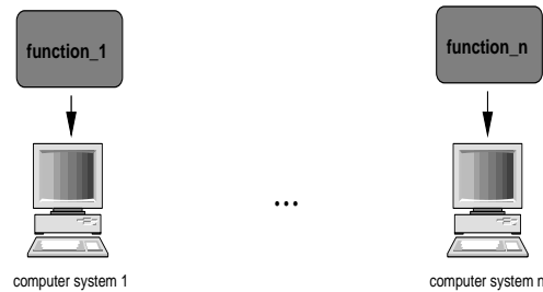
Figure 2: Federated architectures: each avionics function has its own fault-tolerant computers.
