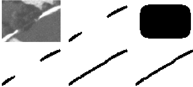
Figure 16: First column: aerial image (© IGN) and the result of extraction using E_0 . Second column: initial contour and final closed contour using the new model E = E_0 + E_{\text{gap}} . Third column: generic initialization and result of extraction with the new model E = E_0 + E_{\text{gap}} . Parameter values: left, [\lambda = 1, \alpha = -0.14, \beta = 0.03, \lambda_i = 2.9, \alpha_i = 0.3, \beta_i = 2.9] ; middle and right, [\lambda = 1, \alpha = -0.14, \beta = 0.06, \lambda_i = 2.9, \alpha_i = 0.3, \beta_i = 2.9, \beta_A = 6] .
