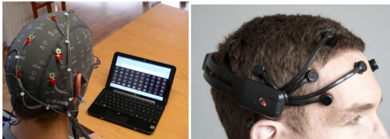
Left: IntendiX running on a laptop and user wearing the active electrodes. Right: dry EEG technologies by Emotiv.
