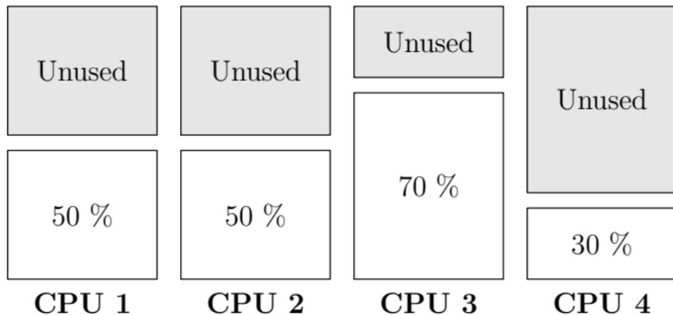
(1) controlling speed of each CPU/core independently
