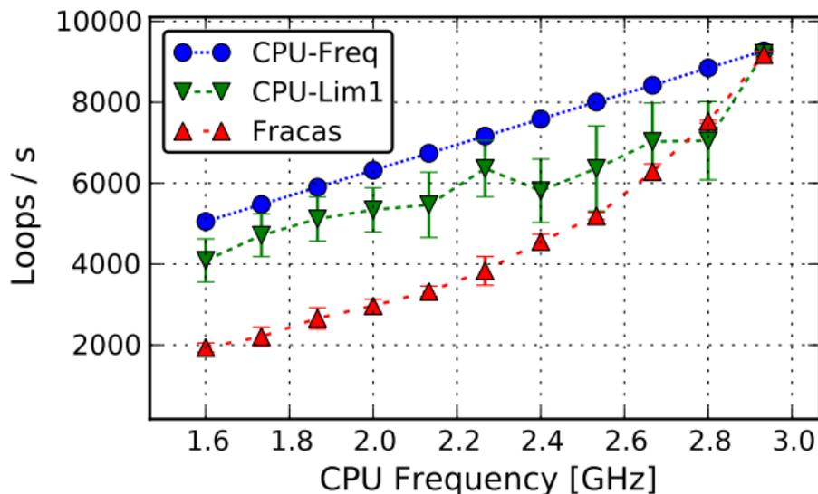
Fracas can't emulate CPU for multitask computation
