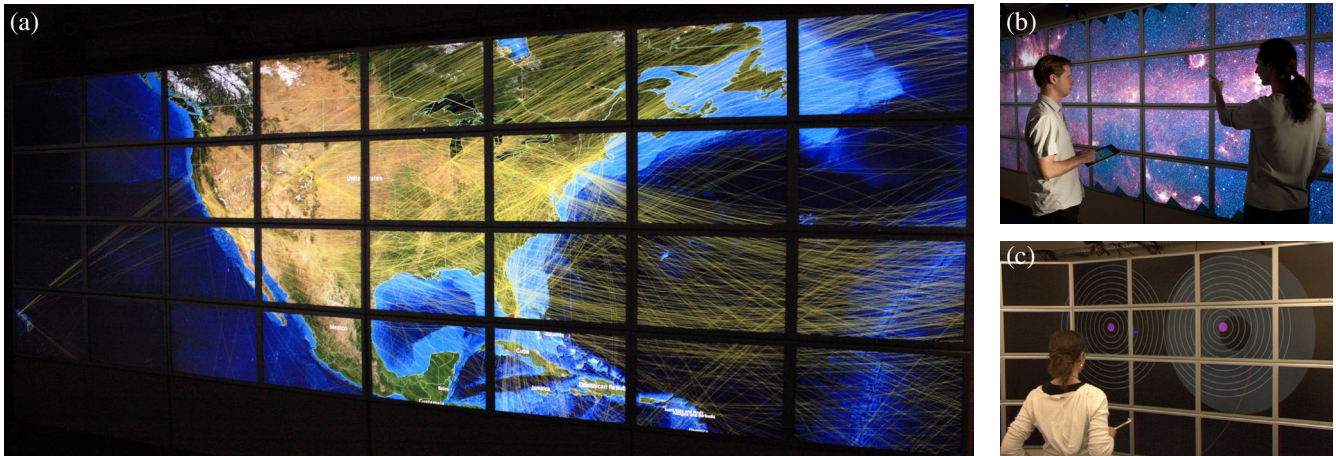
Figure 1. jBricks applications running on the WILD platform (32 tiles for a total resolution of 20\,480 \times 6\,400 pixels). (a) Zoomed-in visualization of the North-American part of the world-wide air traffic network (1 200 airports, 5 700 connections) overlaid on NASA's Blue Marble Next Generation images ( 86\,400 \times 43\,200 pixels) augmented with country borders ESRI shapefiles. (b) Panning and zooming in Spitzer's Infrared Milky Way ( 396\,032 \times 12\,000 pixels). (c) Controlled laboratory experiment for the evaluation of mid-air multi-scale navigation techniques [17].
