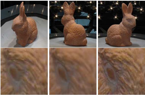
Fig. 1: Top : Multi-view input images for the reconstruction. Bottom left : Close-up of one of the low-resolution input images. Center : Rendered model with blurry texture initialized by weighted averaging of input images. Right : High-quality texture optimized with the proposed superresolution approach.
