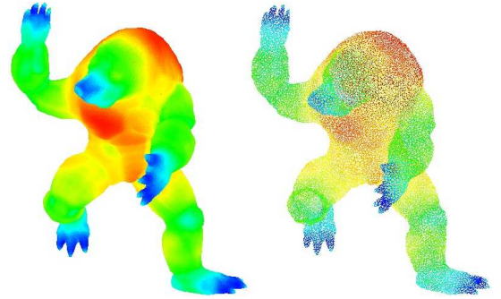
(b) Local error for the Armadillo mesh with facets shrink 40%.
