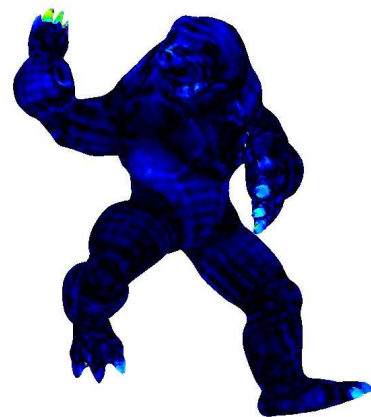
(c) Local error on the Armadillo after 20 smoothing iterations
