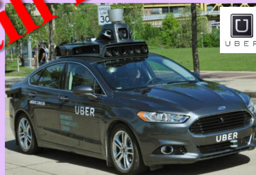
Robot Taxi testing in US (Uber, Waymo) & Singapore (nuTonomy) => Mobility Service , Numerous Sensors ... Safety driver in the car during testing
