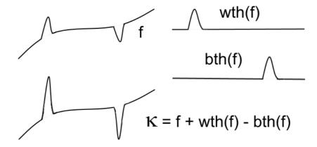
Initial image (upper left), extraction of white features with the white top-hat (upper right), extraction of black features with a black top-hat (lower right), contrast enhancement obtained with the contrast operator (lower left).
