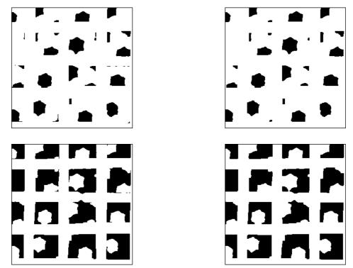
Hexagonal structures extracted by thresholding (upper left), their opening (upper right), background (lower left) and its opening (lower right).
