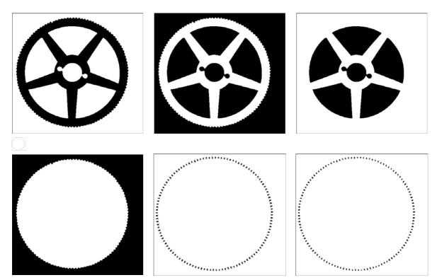
From top to bottom and from left to right: opening of size 3 of the wheel image, negation of the result, removal of the connected component touching the edge (outside of the wheel), difference of the two last images (the outside of the opened comes back), intersection of the outside with the initial image and extracted teeth after a slight filtering.
