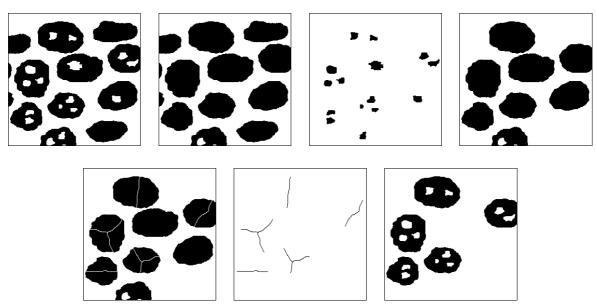
From left to right and from top to bottom: initial image, image with its holes filled, extracted holes, particles with holes (after filling), geodesic SKIZ of the holes in the previous image, boundaries of the SKIZ, geodesic reconstruction of the particles containing at least two holes.
