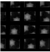
Each background cell is valued with its maximal grey value (left). Subtracting the initial filtered image extracts the hexagonal structures.
