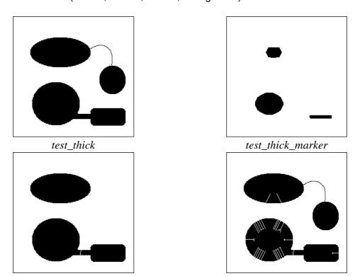
Result of the geodesic thickening when the L structuring element is used (left image) and when the D structuring element is used (right image).
