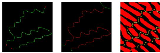
Left: end points (red) of the dislocations (green). Middle: the simple arcs touching the edge and connected to the end points are added. Right: boundaries of the cells containing stacked lamellae.
