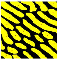
Geodesic centers of the eutectic image (left), centroids (right).
