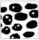
From left to right: particles containing at least one hole, labelled holes, reconstruction of the filled particles with the label image; this reconstruction assigns to each particle the label of only one hole included in the particle. Extracting pixels with identical values in the label image and in the reconstruction produces a mask of the holes to be removed. The result of the filling of a single hole is given in the right image.
