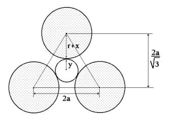
The greater the closing size increases, the more it fills the holes, until they are completely filled. This is achieved when the dilation closes the hole generated by the adjacency of three fibers, that is when:
