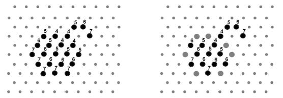
Initial set and its geodesic distance function (left), result of the complete mixed thinning by  $D_3$  double structuring elements (left). The grey points have been removed, but the geodesic distance function is not changed on the remaining points. The new extremities and the geodesic center are still embedded in the previous ones.
