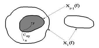
The right connected component of  $X_i$  is a maximum as it cannot be rebuilt by any connected component of  $X_{i+1}$  (it does not contain such a component).
