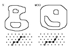
Homotopic transform ( $\varphi(X)$  and X can be superposed without tear) and homotopic paths (the second one can be obtained by a continuous displacement of the first one).
