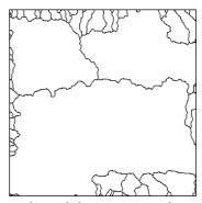
The minima of the filtered relief image are touching the edge of the image and correspond to real outlets (left). Watershed transform of the filtered image (right).
