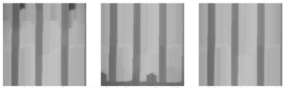
*Vertical closing in direction 1 (left), in direction 5 (middle). Sup of the two closings (right).*
