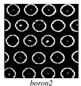
The *boron1* and *boron2* images represent boron fibers in a composite material. These fibers reinforce the mechanical resistance of the material. The resistance increases in proportion of the regularity of the fibers layout. Therefore, during industrial production, they are as far as possible placed according to a regular hexagonal network. However, irregularities occur.
