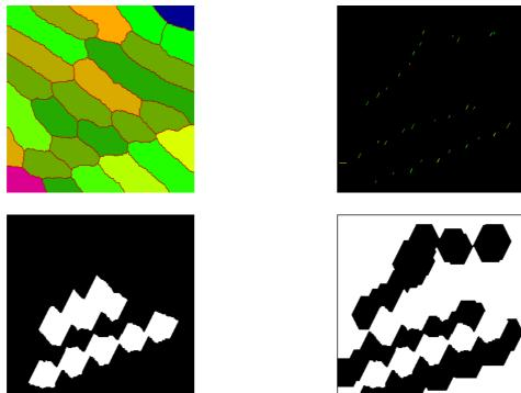
Top left: influence zones valued with half their thickness + 2. Top right: extreme points valued with the previous image. Bottom left: geodesic space used for the adaptive dilation (the separation zones are excluded). Bottom right: result of the adaptive dilation after closing.
