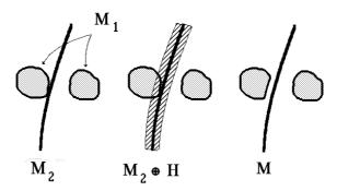
Preventing that markers of the blobs  $(M_1)$  touch the background marker  $(M_2)$  by removing points of  $M_1$  which are inside the elementary dilation of  $M_2$ . M is the final marker set.
