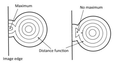
When the parameter edge is set to EMPTY in the computeDistance operator, no maximum appear (right image), whereas this maximum is present when edge is set to FILLED (left image).
