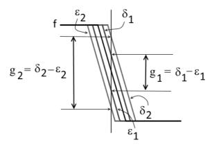
Value  $g_1$  of the gradient when elementary erosion and dilation are used. Value  $g_2$  corresponding to a thick gradient of size 2.
