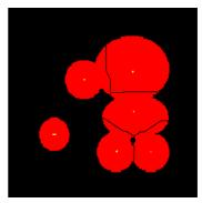
Initial disk image (left) and geodesic influence zones (in red) of the components of the ultimate erosion (yellow).
