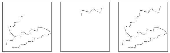
Left: dislocations extracted by the last procedure. Middle: dislocations previously detected. Right: final dislocation extraction.
