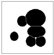
Distance function of the disk image (left), segementation by the watershed of the inverted distance function (right).
