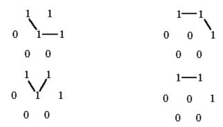
Initial paths before thinning (left) and equivalent paths after thinning (right). The central point has been removed but a path joining the extremities of the initial path can still be defined because the neighborhood points remain after thinning.
