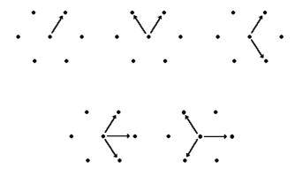
Set of all the configurations where the directional gradient can be maximal (its value is the same for all the concerned directions).
