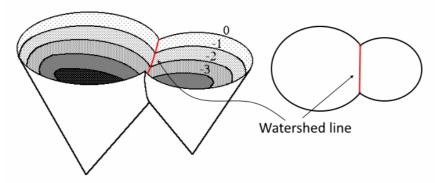
The separation between two particles (right) corresponds to the watershed line of the inverted distance function of the initial set (left).
