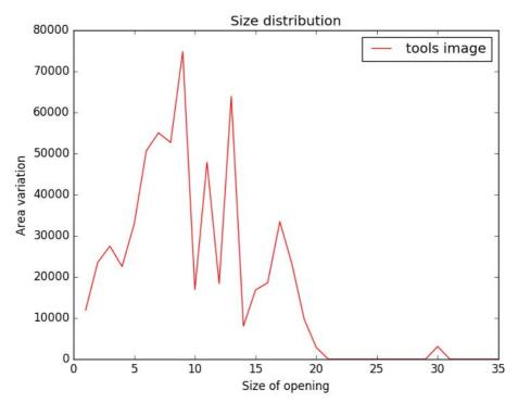
Size distribution of the opening by reconstruction. No variation occurs between sizes 21 and 29. No object has been removed in this range.
