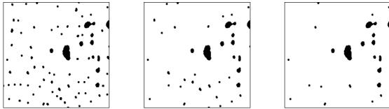
From left to right: minima with a dynamics higher than 10, 50 and 100 extracted from the filtered electrop image.
