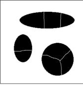
The geodesic SKIZ of the holes does not produce necessarily multiple points when the number of holes is greater than 2 as illustrated in this example. Upper left: initial image. Upper right: geodesic space (initial image without holes). Lower left: holes. Lower right: geodesic SKIZ of the holes in the geodesic space.
