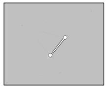
Consider the set X made of two connected components. The geodesic space is the entire field minus X. The set to be thinned is the set Z\X. Performing a full geodesic thinning using all the directions of the homotopic structuring elements until idempotence produces a connection between the two initial connected components.
