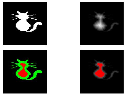
Initial set (upper left), distance function computed on the hexagonal grid (upper right), erosion of size 12 of the initial set (in red, lower left) and section at level 13 of the distance function (lower right).
