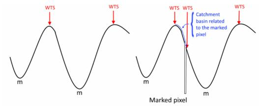
A new source of flooding is created at a specific position by simply replacing the pixel value by 0. A well is generated. When the flooding coming from the other source included in the same catchment basin reaches the point, a new watershed line appears, delimiting the catchment basin related to the point.
