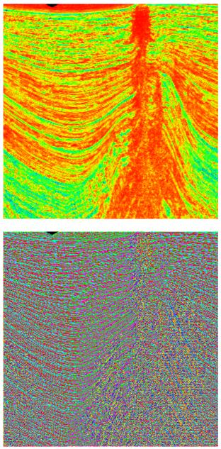
Gradient modulus of the seismic\_section image (top), gradient azimuth (bottom).
