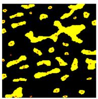
Geodesic centers (in red, after a dilation) of the metal1 image (in yellow) obtained by the geodesicCenter operator.
