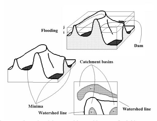
The topographic surface (left image) of the initial function is flooded from its minima. Merging lakes are separated by a dam (upper right image). When the process is complete, the image is partitioned in catchment basins containing one minimum separated by the watershed lines (lower right image).
