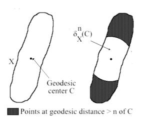
The successive geodesic erosions of the set  $X\setminus C$  (or geodesic dilations of C) correspond to successive levels of the geodesic distance function.
