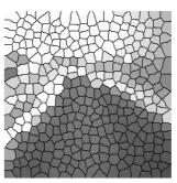
The maximum value of the road1 image (left) in each cell of the tesselation image (middle) is used to label it (right image).
