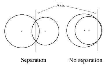
The separation of two disks by ultimate erosion fails when the disks are too intricated. The limit condition occurs when their centers are on the same side of the radical axis.
