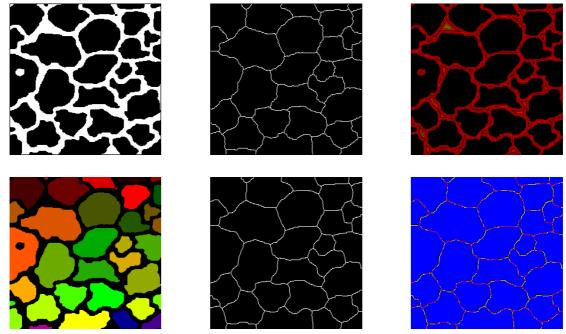
From top to bottom and from left to right: initial alumine image, SKIZ obtained by thickenings, distance function of the complementary initial image, labelling of the initial image, SKIZ obtained by watershed of the distance function, comparison of the two SKIZ: apart some local variations due to different choices of initial directions of propagation, the two SKIZ are similar.
