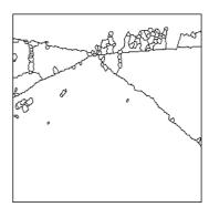
Initial road image (left). Highest level of hierarchy (4) with a gradient of size 1 (middle). Highest level (3) with a gradient of size 2.
