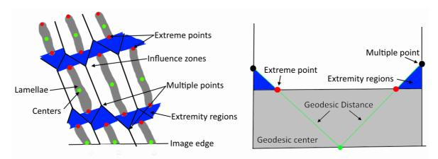
The geodesic centers and the extreme points of the lamellae are extracted. The geodesic distance of the centers inside the influence zones is computed. The influence zones are labelled with the extreme points and are assigned the maximal distance of these points inside each influence zone. The mask of all the points where the geodesic distance is higher than or equal to the labelled image defines the extremity regions.
