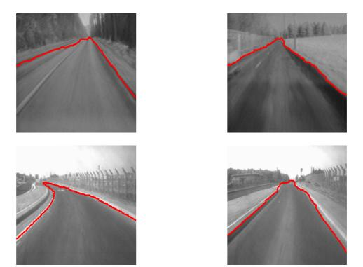
From top to bottom and from left to right, result of the road segmentation algorithm applied to the route, road, road1 and road2 images.
