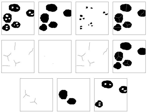
From left to right and from top to bottom: initial image (particles with at least two holes), particles without holes, holes, geodesic SKIZ of the holes, boundaries of the SKIZ, multiple points, simple arcs of the SKIZ, second geodesic SKIZ of the simple arcs, boundaries of the second SKIZ, reconstructed particles (particles with more than two holes), final result (particles with two holes).
