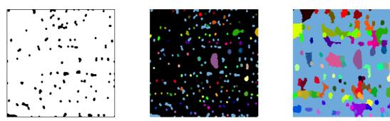
Maxima of the initial filtered image (left), label image where all the maxima have the same label (middle), result of the gradient watershed (right).
