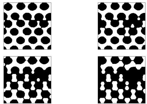
From left to right and from top to bottom: closings of increasing sizes (4, 6, 8 and 10) of the boron fibers.
