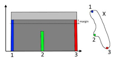
The particle X has 3 extremities. In light grey, indicator function of X. In dark grey, result of the geodesic reconstruction of the indicator function by the valued extremities. The extremities 1 and 3 are at the same height as the reconstructed image. The margin parameter allows to select extremities at a lower height.
