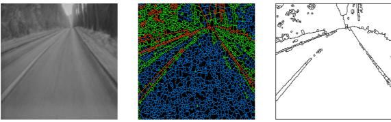
Initial route image (left), result of the enhanced waterfalls segmentation, each level of hierarchy is represented with a different color (middle), extraction of the highest level of hierarchy (right).
