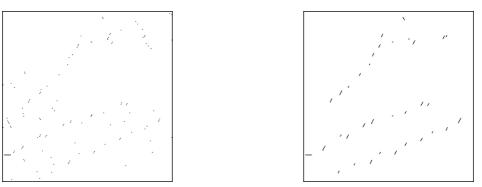
Extremities of the eutectic image (maxima of the geodesic distance) on the left. On the right, extremities of the same image after an opening.
