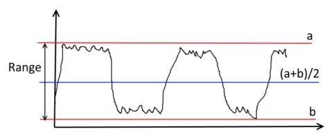
Principle of the automatic thresholding of a two-phased image; the extremal grey values a and b are computed and a threshold can be applied in the middle of the range.
