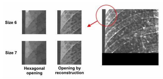
Difference between the hexagonal opening and the erosion-reconstruction opening observed on the left feature (red circle) in the lung2 image. The evolution between sizes 6 and 7 is progressive in the case of the hexagonal opening (the white feature size decreases gradually), whereas it is sudden with the erosion-reconstruction opening.
