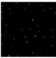
Geodesic centers obtained with the geodesicCenter procedure in yellow, with the thinD in green (centroids). When both centers are superposed, they appear in red.
