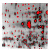
Minima (right) of the electrop image (left) filtered with an alternate sequential filter of size 2 starting with an hexagonal opening.
