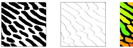
eutectic image (left), its horizontal intercepts (middle) and labelling of each connected component with its vertical diameter (right).
