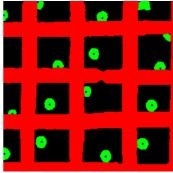
Restriction to the spots of the distance function of the union of the spots and the raster (left). Spots in green, raster in red and centers of the spots in blue (right).
