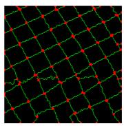
Watershed transform of the inverted steel\_sheet image (left) and its multiple points (right).
